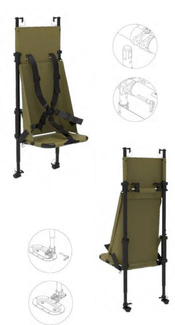
T-MAK crashworthy seats absorb ground impact energy by stroking downward relative to the aircraft floor at a load which is preset to approach the upper limit of human spinal compressive tolerance.
