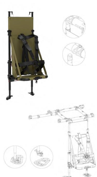
T-MAK crashworthy seats absorb ground impact energy by stroking downward relative to the aircraft floor at a load which is preset to approach the upper limit of human spinal compressive tolerance. Wearable restraint system provides movement ability.
