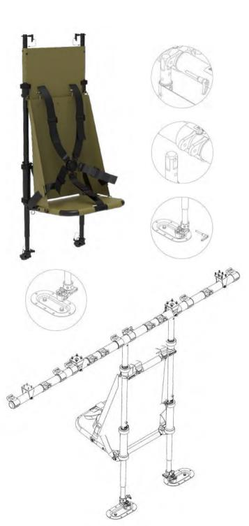
T-MAK crashworthy seats absorb ground impact energy by stroking downward relative to the aircraft floor at a load which is preset to approach the upper limit of human spinal compressive tolerance.
